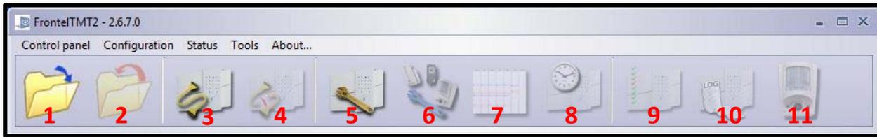
1. **Open Alarm Panel List:** This shows all panels that have connected to this TMT Installer in the past. If a panel in that list is currently connected with the PC and transmitting an event to the panel it will have a check mark next to it. To OPEN the panel, click on the serial number and hit the OK button
